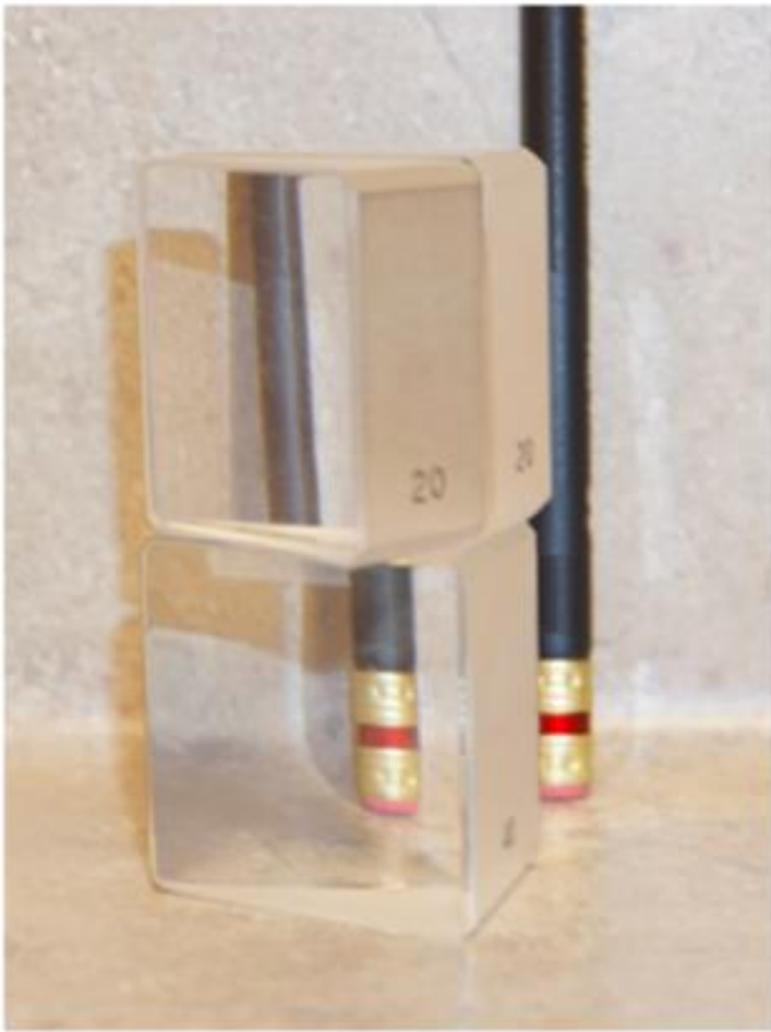
Fig. 2.2 On the bottom is a 40 \Delta prism. On top of that is a sandwich of two 20 \Delta prisms. The top prism sandwich has a much greater value than the 40 \Delta prism, as evidenced by it displacing the image of the pencil much further
